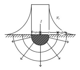
Fig. 1. Hemispherical ground body and its potential distribution in homogeneous soil
